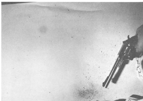
FIG. 2—Placing the weapon back in the original position after the shot. The relationship of droplet size versus distance traveled can easily be seen.
